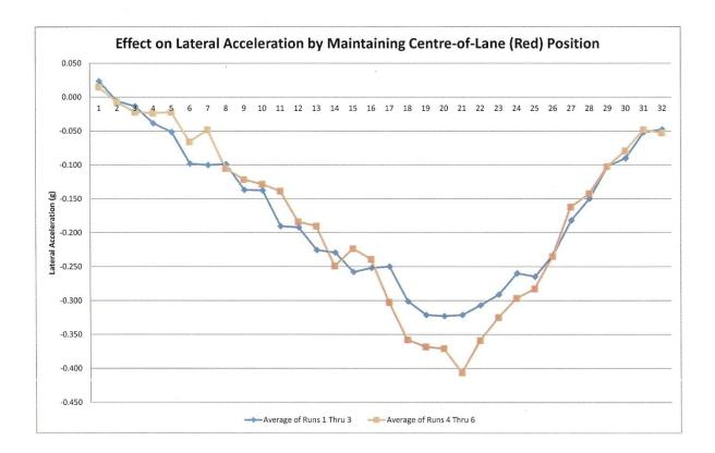
The blue line represents the average acceleration from three tests where the test driver simply followed the normal procedure for passing through the curve by steering close to the centre-line near the beginning and then allowing the vehicle to drift toward the outside (right) portion of the lane in the latter part of the curve. As seen in the table the maximum lateral acceleration of over 0.3 g was substantial.
